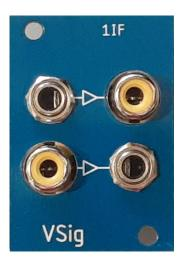
1IF InterFace is a 6HP 1U tile for buffered interfacing between RCA connected 75-ohm video and standard eurorack 1V video signals. Converters for both directions are provided: from RCA to eurorack, and from eurorack to RCA.
