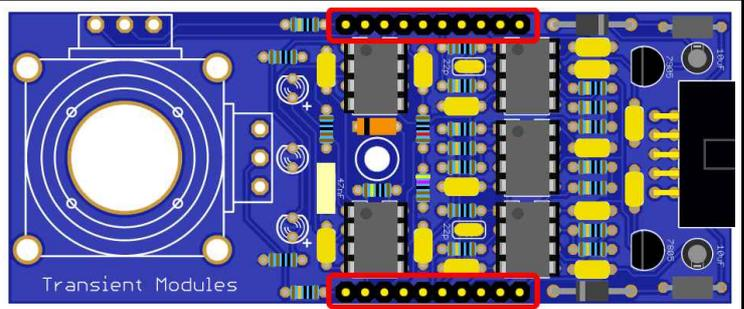
20. Now the top board. Solder the 3 remaining resistors: 1K, 470K, 100K.
