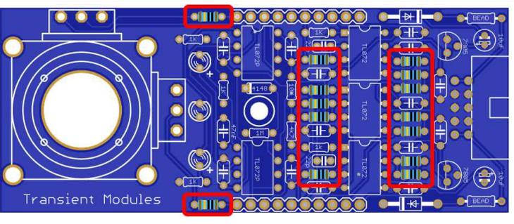
3. Solder the 1x **10K** resistor.
