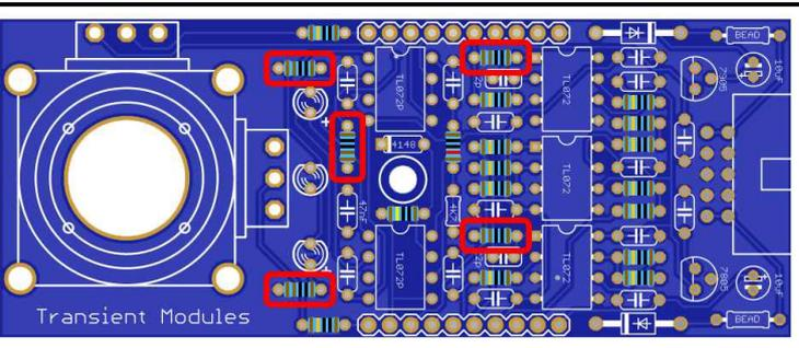
6. Solder the 1x **4K7** resistor.
