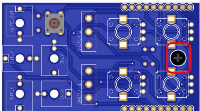
23. Solder the 2x 10 pin female header ensuring they're both 90° to the PCB.
