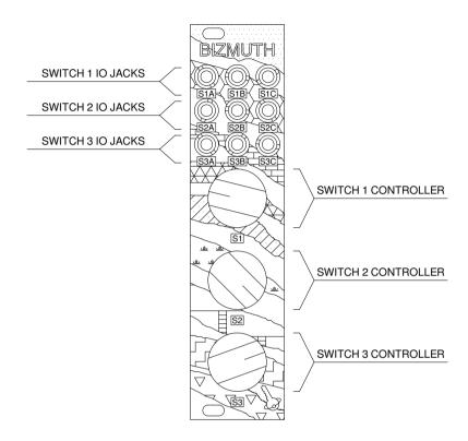
Bizmuth is a gesture based chaotic signal router and gate generator. You can route switch or combine up to six signals, or generate up to six gates by turning three endless knobs with one hand. Small tweaks can have large effects on routing or gates, giving the module a very tactile and chaotic feel. If you are into noise, glitch, sound design, or chaos, Bizmuth is a great tool for you on stage or in the studio.
