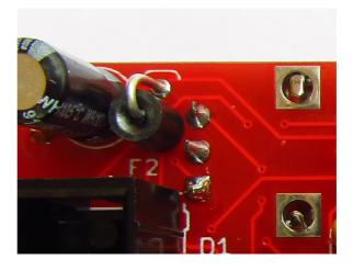
If the ferrite bead sticks out too much, slightly press on them with your finger (or thumb) and reheat the solder. When they are correctly placed, solder the other leg.
