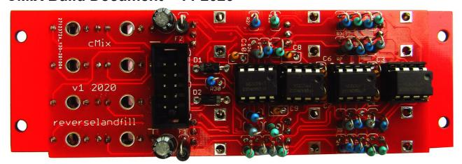
This pcb is quite dense, as most parts are placed 'standing up'. Because of this, the order of placing parts is important. Start with the lowest parts!
