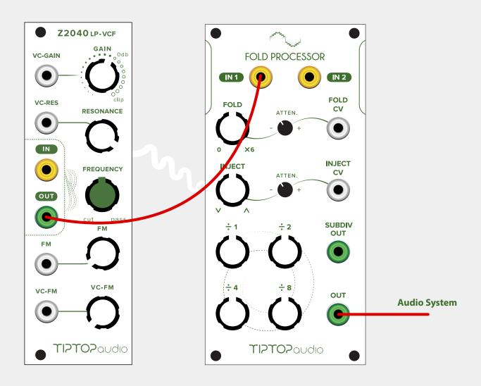
To get started patch as the drawing above, set your Z2040 resonance to max, set the frequency knob half way, this will cause the Z2040 to self oscillate a natural sine wave (if you don't have a Z2040 use the sine output from your Z3000). Plug the Z2040 out into the IN1 on the Fold Processor (we'll call it just Fold from now on). Connect the Fold OUT jack to your speaker system and sweep the FOLD knob, if you don't hear a sound change the INJECT knob as it might be in the 'dead' zone.
