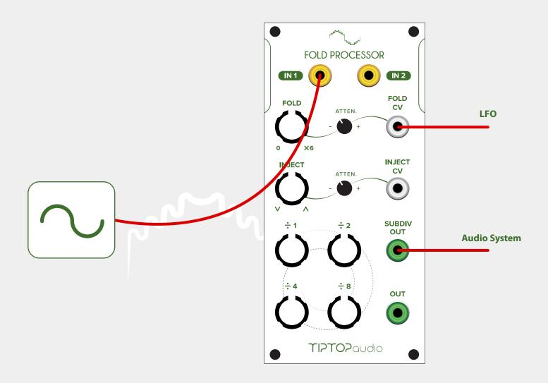
The subdivide circuit gets totally wild when sweeping the Fold and Inject knobs, octaves move in and out and pulses get pulse width modulated. The sound ranges from sweet at times to total destruction at others; experiment by adding some delay from the Z-DSP and things get really interesting.
