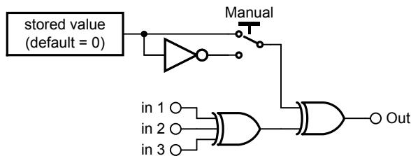
Xor can be used as a “digital ring modulator” such as implemented in the ARP Odyssey and KORG MS-20 synthesizers. Feed two inputs with two oscillators to get the effect.
