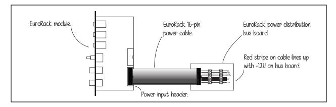
After connecting the power cable, mount the module frontpanel flush to your enclosure's EuroRack mounting rails and secure the module with the mounting screws provided by your enclosure's manufacturer.
