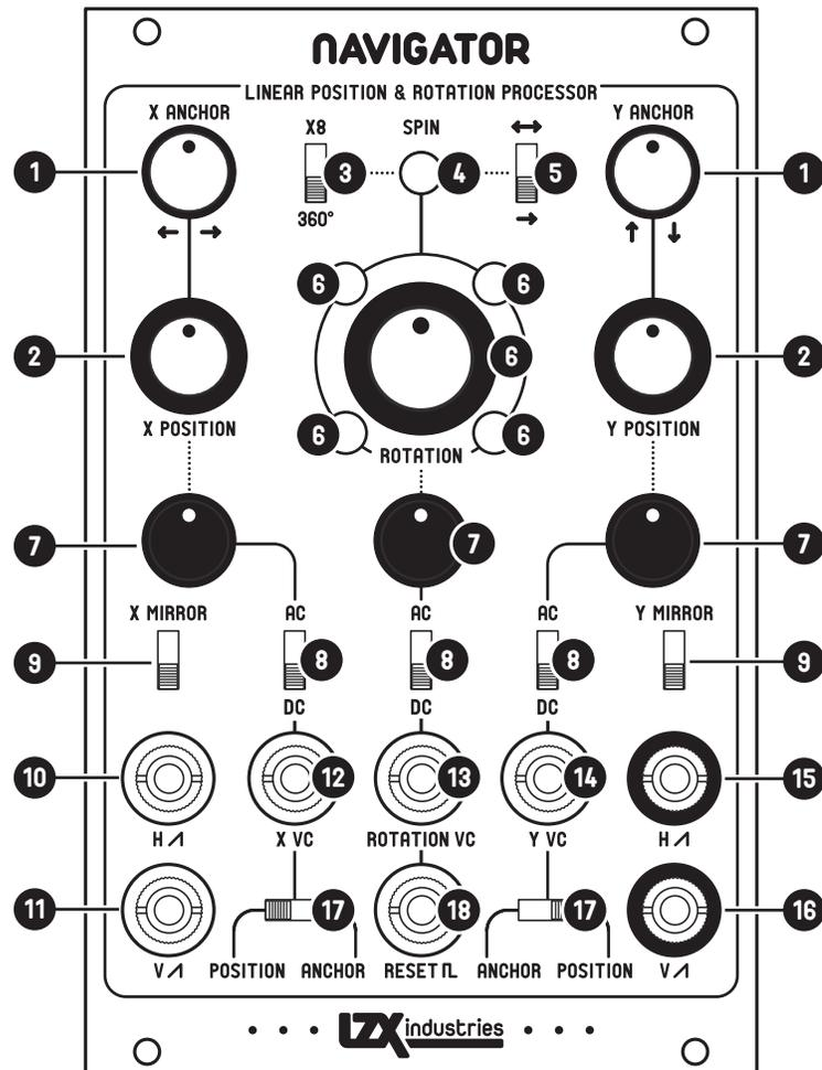
**12** X position voltage control input. 0-1V DC full scale. The depth of modulation is set by the associated inverting level control.
