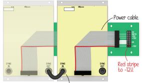
RCA cable connects sync output from system's video sync generator (or daisy chained module) to sync input on rear of module.
