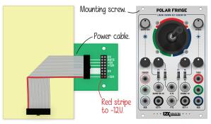
Mount the module in your case using the mounting screws provided by your case's manufacturer.
