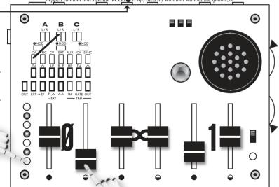
\*Set all faders at max. \*Press and hold REC button. \* Release REC and enjoy the max blast.
