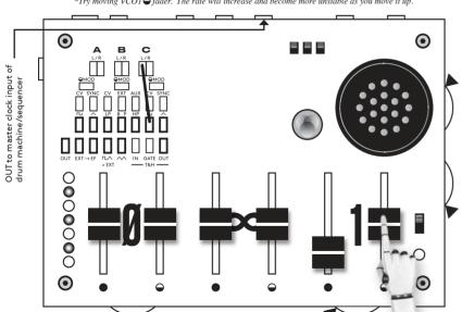
\*Connect clock signal from drum machine to VCOI sync socket via the jack adapter
