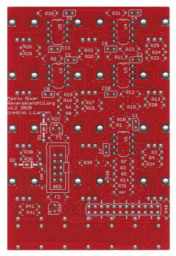
The Matrix mixer is designed for use with a LZX format modular videosynthesizer. Use it for color routing, mixing and inverting several sources, feedback patching and softkeying. There are several MOD options, such as gain amplification and external 'overall gain' potmeters.
