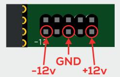
Now take a multimeter and check if there's no shortcut between the ground, 12V and -12V pins on the power header. If nothing's wrong, you're good to go! Plug the power cable and make sure the red stripe of the cable matches the -12V on the PCB silkscreen. Don't forget to add the nuts on the connectors, switches and potentiometers, finally add the knobs. Now let's plug the module in your system and test it. The module
