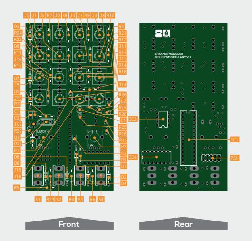
The front of the PCB is the one with the switches, jack connectors and potentiometers on it. The top of the board is the connectors side, the bottom is the switches side. Almost all the components goes to the front of the PCB. Here is a list of the components that goes to the rear side :
