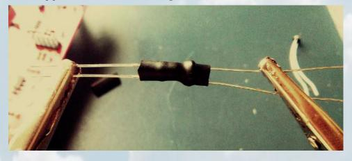
Put the vactrols on the IDC pins as on the picture below:
