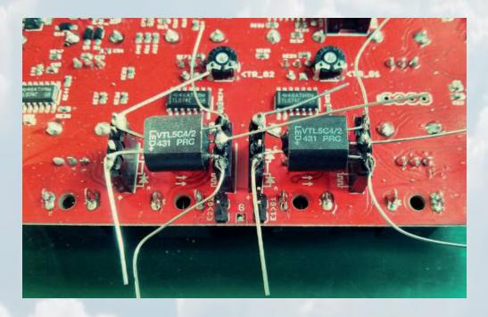
LED's legs (in case dual vactrol) should be soldered to the most upper and bottom pins. Two middle pins of each socket are
