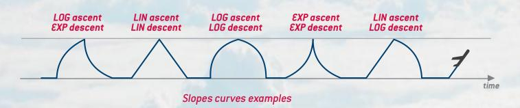
The CV Input for each Airplane's stage requires **3.5 mm mono plug (not stereo)** to function properly. The range of acceptablevoltage is  $\pm$  5 volts (10 Vpp). It's also possible to contol the shape of the slope (from exp-to-lin-to-log) instead of the time. By installing appropriate jumper settings (see the **Jumperization Chart**) the control of the input voltage is changed from 'control over parameter time' to 'control over parameter shape'.
