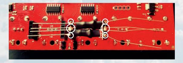
After soldering, cut all the long legs cut from the vactrols off so they will not connect somewhere else.
