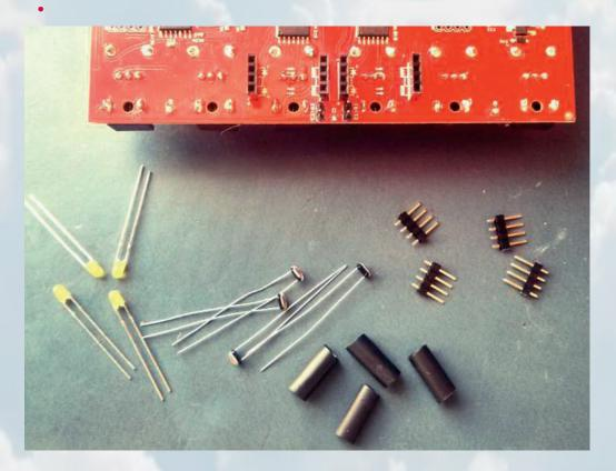
Same as in chapter 1 – you need to prepare 2pcs. of PLS-4 4-pin strips for each Gate. Additionally you need to prepare 2 pcs. of black 1cm length heat-shrink tube per each Gate.
