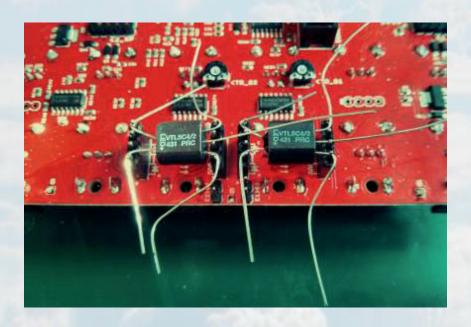
The factory vactrols should be put with their wires between the IDC pins with the graphics labeled upside up. The side with two LED pins (labeled as LED+ on the vactrol's case) should be on the left side of appropriate socket (LED+ on the vactrol should be on the same side where + is marked on the PCB).
