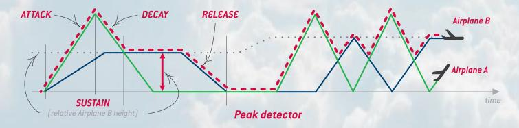
In *looping* mode both Airplanes work as *Voltage Controlled Oscillators* with *separately controlled* take off and Landingslope rates as well as *separately controlled* shapes of each slope. The take off and landing knob in far counterclockwise position, with no additional voltage applied, each stage has a duration of 1 ms or 500 Hz per whole cycle.
