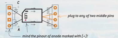
Before installing the opto-couplers you may want to cut their legs off to 1 cm length each and bendthem 90° down to fit into socket. After installing new opto-couplers and checking the gates are working properly, you may apply a small amount of hot glue to the spots where the pins are inserted into the sockets to ensure the opto-couplers will stay there firmly.
