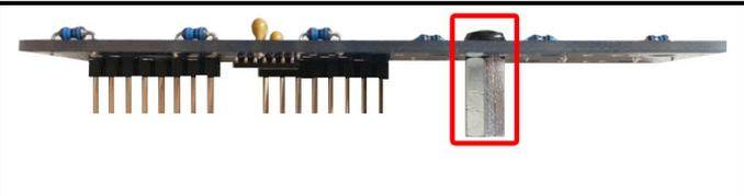
18. Place the **6x jack sockets**, the **3x 100KB potentiometers** and the **3x leds** into their position but **DO NOT SOLDER** anything yet.
