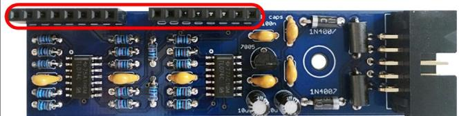
11. Now the top PCB! Start with the SMD parts again. Solder the 1x **TL074**. Position it with **the line on the top face** of the TL074 at the same end as **the circle (pin1) in the silkscreen**, as shown in the image.
