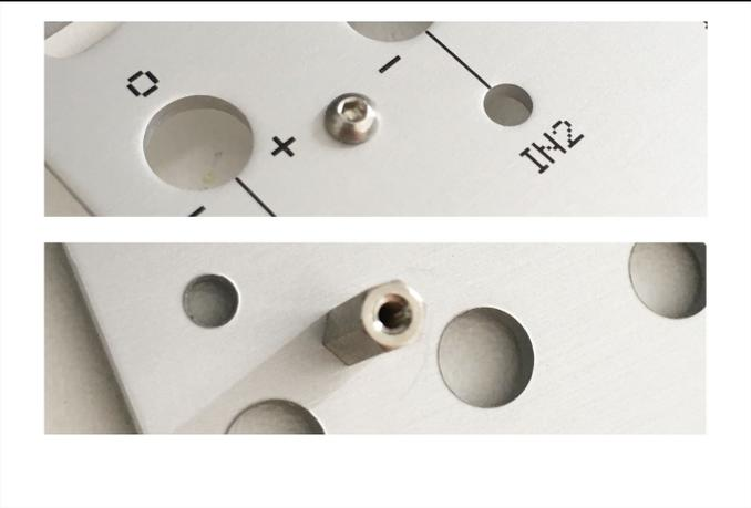
20. Place the front panel moving a little the parts if necessary. The spacer in the panel should match the hole in the PCB. Join both using the **phillips M2 screw**.
