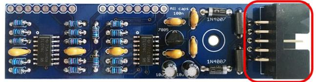
10. Solder the 2x **8 pin female header**.
