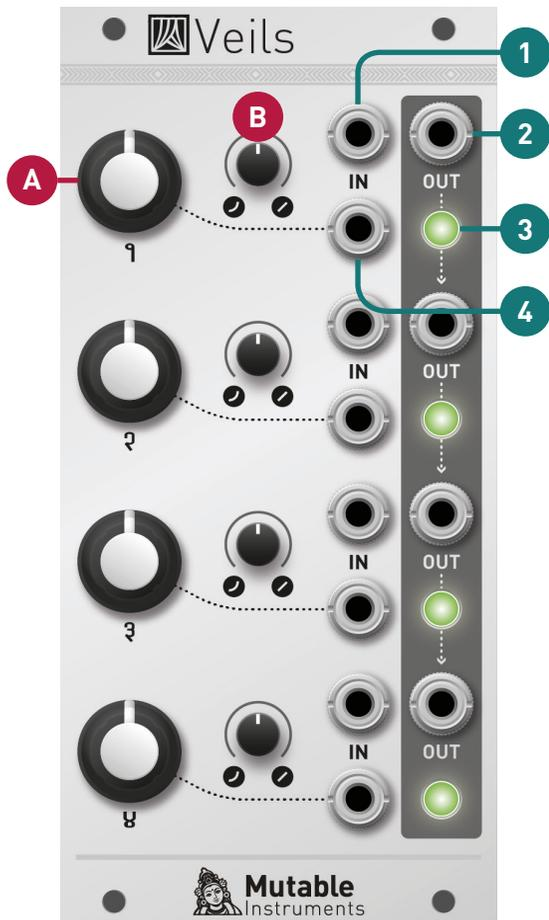
**A. Gain CV amount.** Amount of gain (amplitude) modulation from the CV input (4), or direct gain control when no cable is patched in the CV input. When this knob is turned fully clockwise, a CV of +5V yields a gain of 1, and a CV above +5V might cause distortion.
