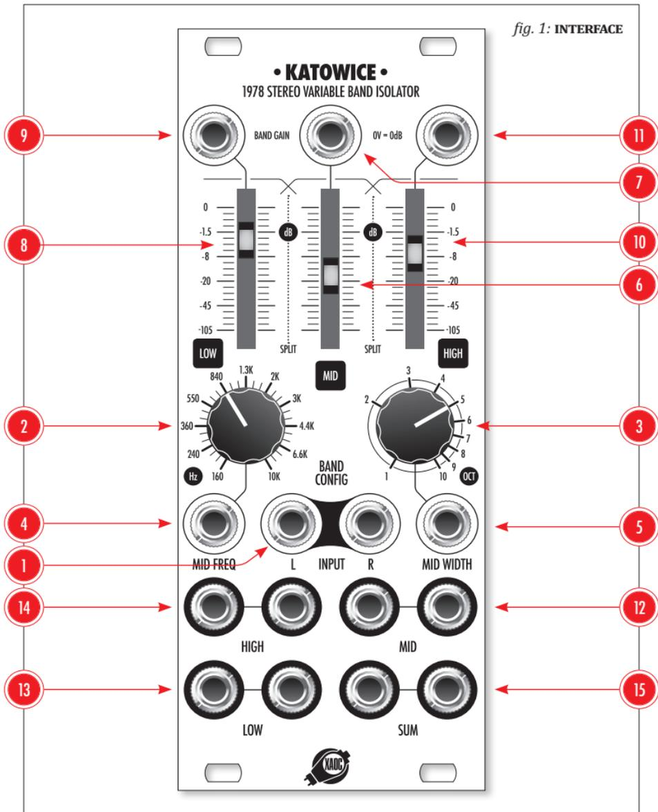
quencies, and the right **HIGH** slider 10 and CV input 11 control the high frequencies. The middle band signal is available at the stereo pair of **MID** outputs 12. Similarly, the low band and high band are available at their stereo pairs of **LOW** and **HIGH** outputs 13 and 14. A stereo mixdown of the three bands (post-VCA) is available at the **SUM** pair of outputs 15.
