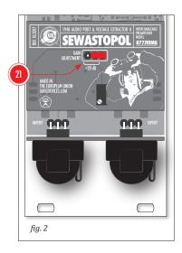
a 6.3mm (1/4") plug to the IMPORT jack and carefully set the gain. The preamplifier accepts very weak to very hot signals and features high input impedance (10M0hms) so that it sounds great with coil and piezoelectric transducers. It offers a gain of up to +60dB on the knob plus an optional boost of
